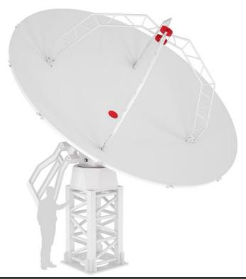
INTREPID 500-20 features a precise 5.0m solid dish antenna capable of recording frequencies up to 20 GHz, and GS-800II antenna tracking system with N-ACU Next generation Antenna Control Unit for high-precision tracking, remotely controlled with fast slew speeds (up to 19°/sec) and elevation axis flip to avoid any keyhole effect. INTREPID 500-20 can be used with third party frontends and backends or it can be equipped with S/X Dual-Band Coaxial Feed for L, LHC and RHC polarization.
