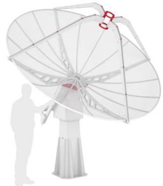
INTREPID 300-5 is composed of 3 meter mesh dish antenna, high precision GS-100II antenna tracking system and C106-HEAVY pier for concrete base. Special design of the mount with high-torque motors, coupled with gear box, offers a perfect structure mechanical balance and a wind survival speed of 150 km/h.
