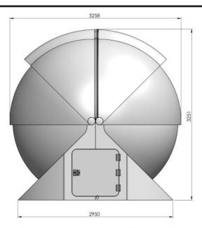
Constructed with a multi-layer GRP (Glass Reinforced Plastic) structure and featuring anodized aluminum and stainless steel components, the OUTPOST 3M delivers enhanced rigidity and durability, ensuring long-term stability even in the most demanding environments. High-speed motors and advanced remote-control electronics guarantee rapid opening and closing, while a selective shutter mode allows partial opening to protect the telescope from strong winds without sacrificing visibility.
