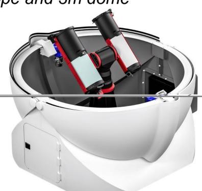
DUAL-PRO includes a very high precision and load capacity alt-az mount with heavy pier that supports 2 telescopes in parallel: a wide field telescope and a higher magnification one, both with robotic focusers, ARCO rotators, GIOTTO flat field generators and ALTO telescope cover motors. Every telescope comes with a special camera, this way the user is able to take pictures of the same object at different magnifications.
