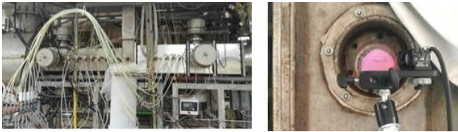
Fig. 9 Atmospheric burner test rig and cooled window for camera installation
