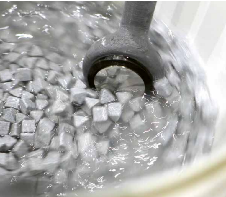
Slurry pot with abrasive medium in artificial seawater (3.5% NaCl solution).
