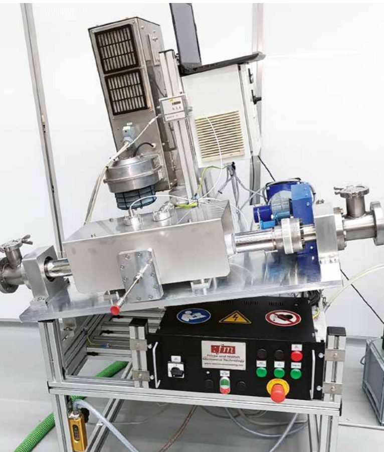
Microwave pyrolysis system developed within the "PV-Kreis" project.
