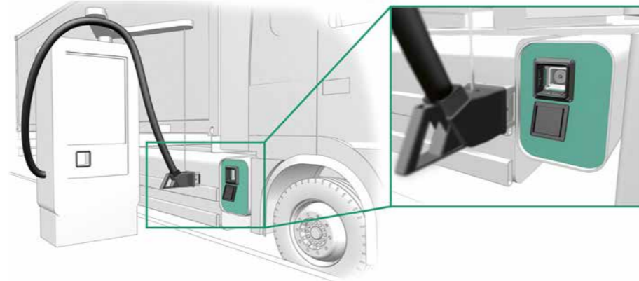
1 Charging system for e-mobility based on a novel form of face contacting.
