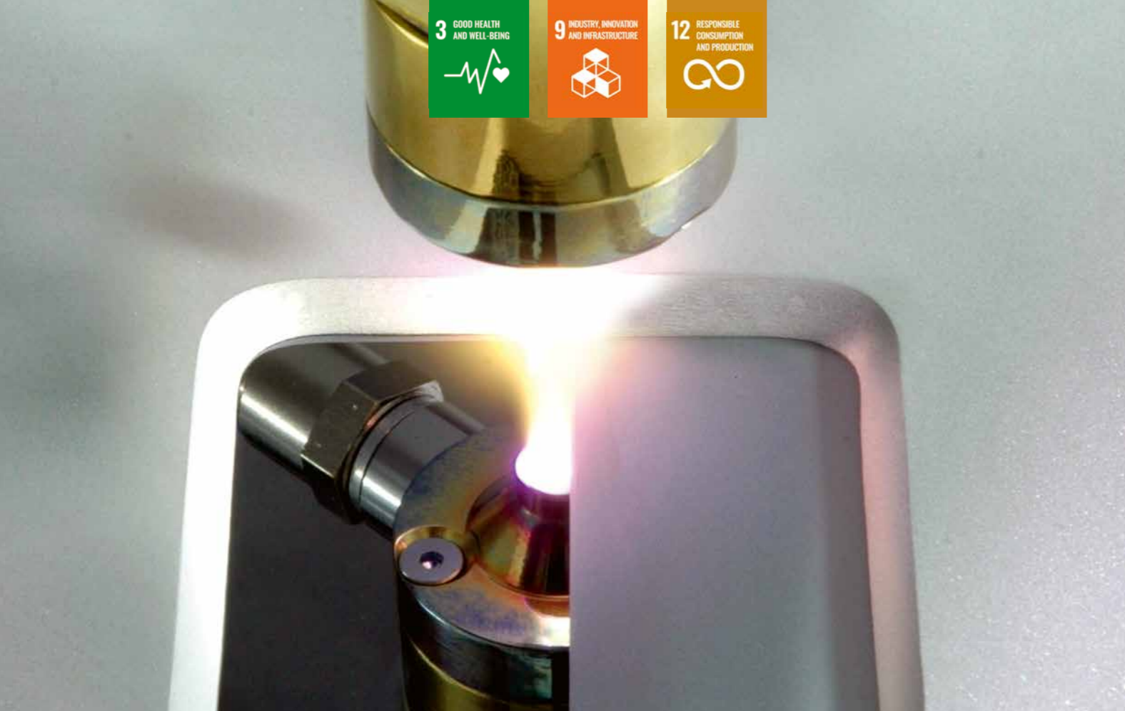
Via the side-mounted nozzles, a multitude of powders can be introduced into the plasma jet.
