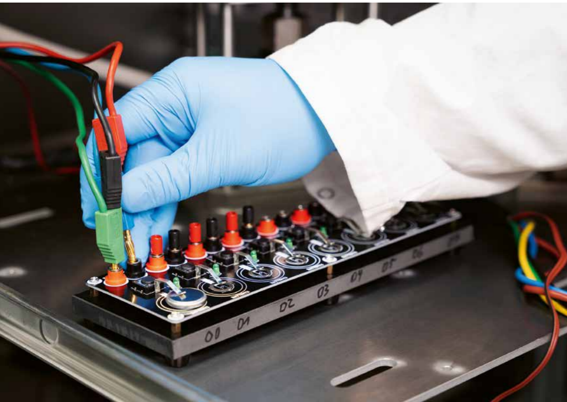
Preparation of electrochemical measurements of new materials in button cells.
