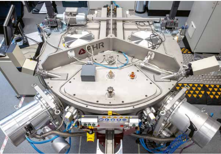
Application of inline measurement technology for the determination of layer-thickness dependence, e.g. of SnO 2 on C60, as well as for the analysis of the time lag occurring at the beginning of the SnO 2 deposition.
