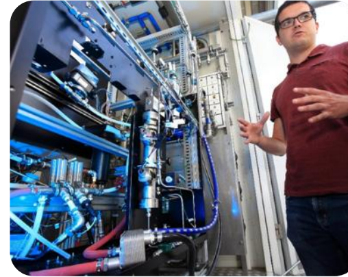
20 kW Stack Test Bench
