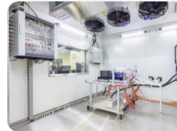
Fuel cell system test bench
