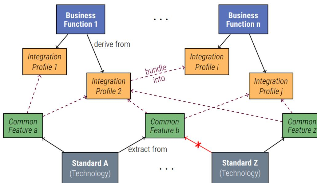
Figure 6: Profile Bundling and Common Features: avoid redundant specification
