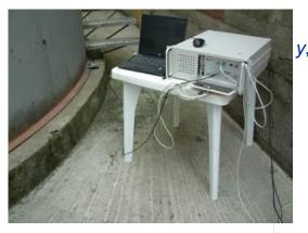
Ultrasonic non-destructive testing of condition of petroleum tank bottom plates in oil and gas sector. No emptying and cleaning of the tank is required!
