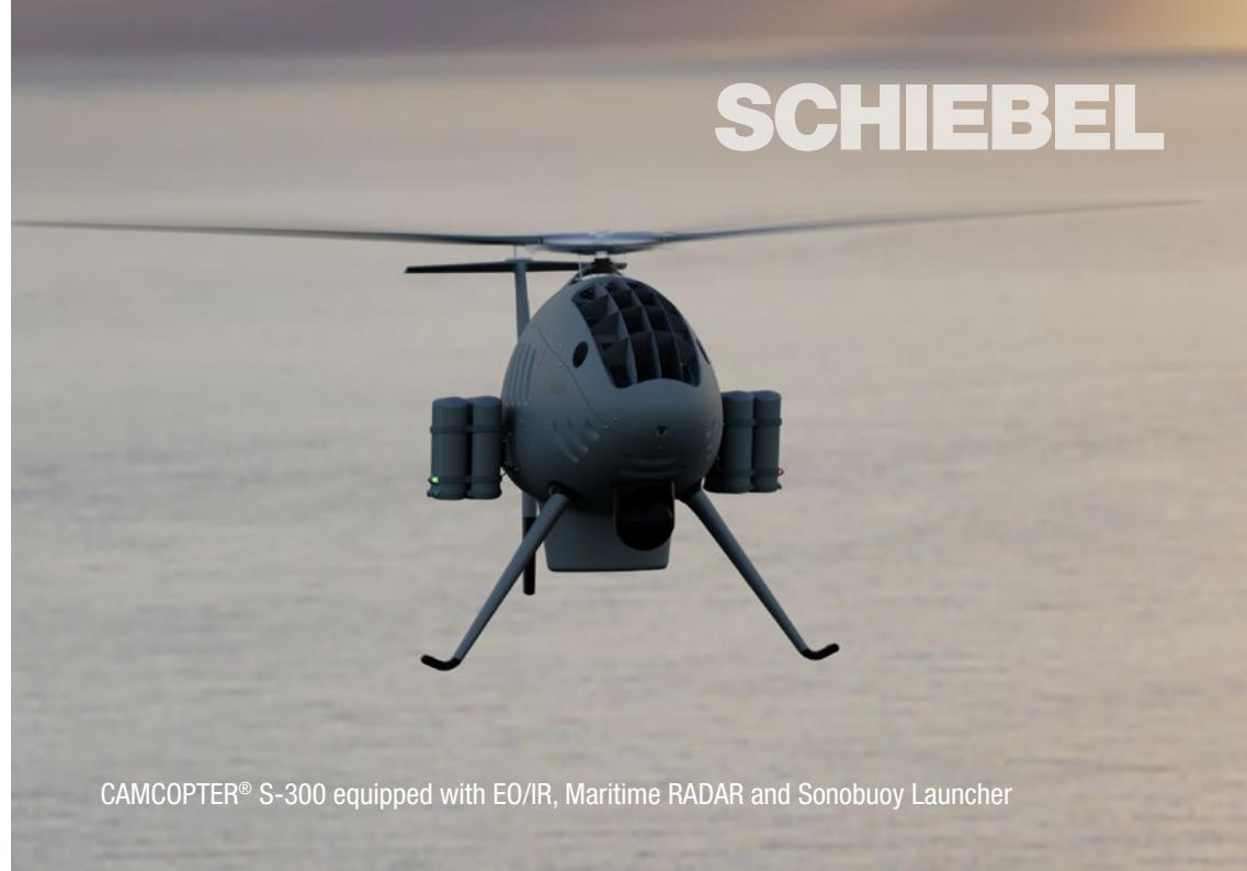
CAMCOPTER® S-300 equipped with EO/IR, Maritime RADAR and Sonobuoy Launcher
