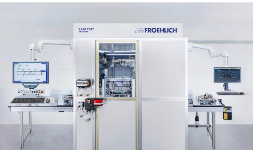
Leak test stand for inverter & power units
