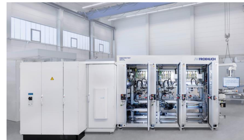
EOL function test for inverter & power units
