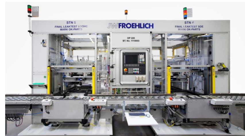
Leak test stand for fuel and hydraulic components
