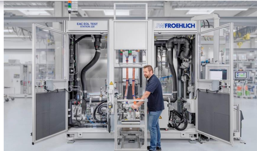
Functional test station for turbine compressor units
