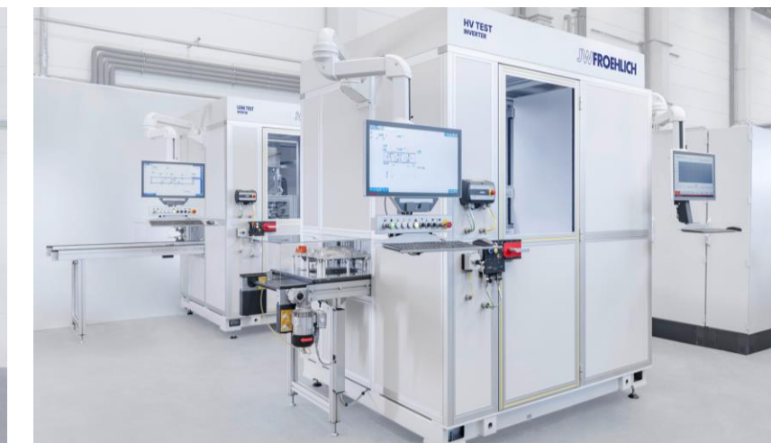
HV test stand for inverter & power units
