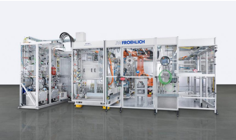
EOL test stand for hybrid units (drive)
