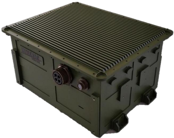
5kWh Li-Ion IP65, MIL-STD-810, MIL-STD-461, MIL-STD-1275 -40 ile +60°C Operational Temp. 5kW Discharge Rate <1,5h Charge Duration RS-485 Communication Protocol Rack Cabinet Compatible For Jammer On Vehicle
