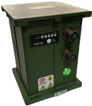
28.8V 8Ah Li-Ion -40 ile +60°C Operational Temp. 5kW Discharge Rate <1h Charge Duration RS-485 Communication Protocol For weapon System
