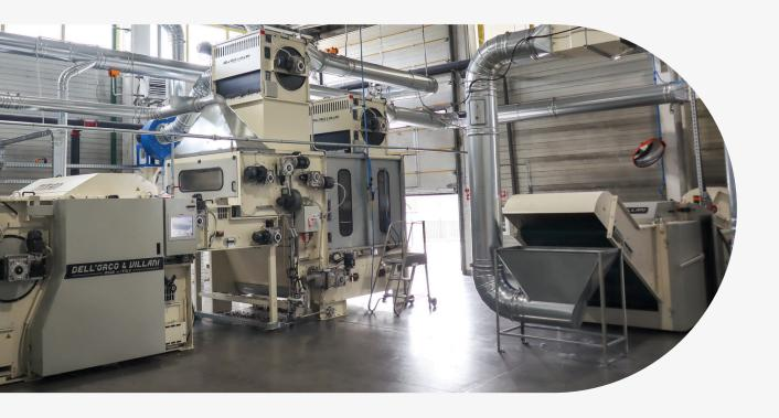
Our full-scale mechanical recycling facility has an estimated capacity of 8000 tons per year. The machine is of a new generation and allows efficient recycling with minimal pollution. We are able to treat the input feedstock to produce frayed fibres as output that can further be processed to variety of non-woven end products and regenerated yarn.
