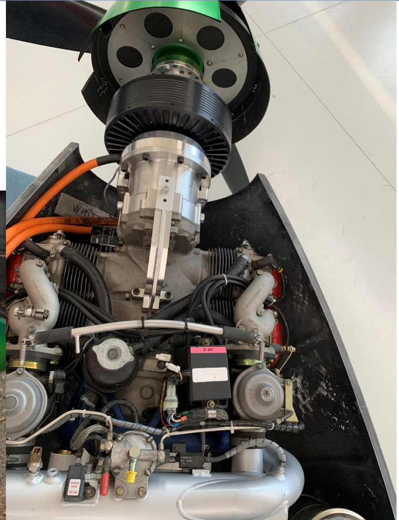
Side view and top view of the hybrid power unit installation on the Dardo
