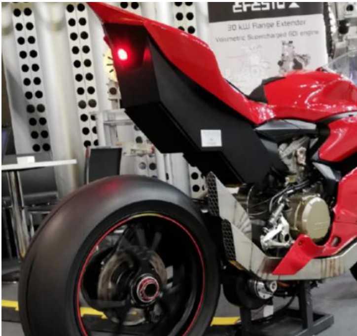
View of the High voltage battery pack developed for the Efesto hybrid motorcycle presented at Eicma 2019.
