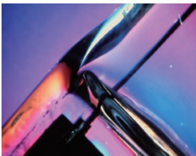
View of measurement of strain on sealing area of FPD by SF-IIC
