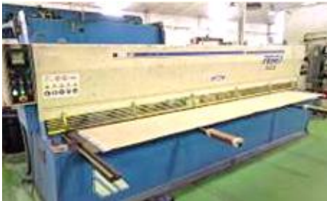
FERRY BBB Metal Shears Effective dimensions: 4150mm
