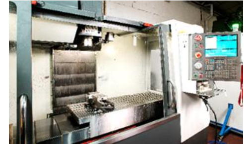
HAAS VF4S 3 axis CNC Machining Effective dimensions: 1000x500mm
