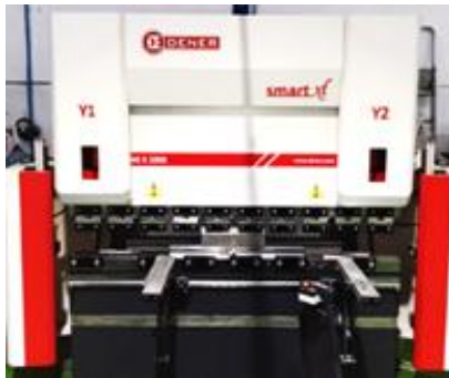
DENER 60TN Bending Machine Effective dimensions: 2000mm
