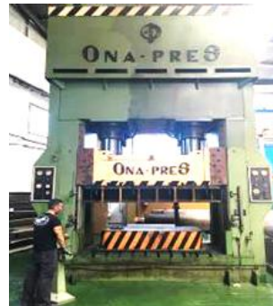
ONAPRES Rubber Press 1200 TN Effective dimensions: 1900x900mm
