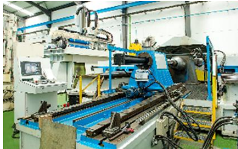
DENN Metal Spinning Fuel tank dome length: 1850mm Diameter: 262mm - 595mm Wall thickness: 12mm
