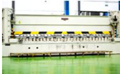
HAEUSLER Roll Forming Machine Effective dimensions: 6000mm
