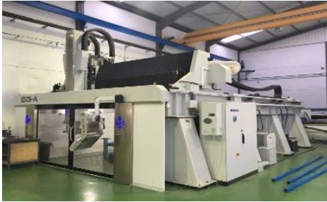
BERMAQ 5 axis CNC Machining X=3000mm; Y=6000mm; Z=1500mm; C(245°), A(120°)
