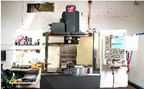
HAAS VF4S 3 axis CNC Machining Effective dimensions: 2000x510mm
