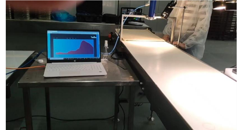
In-line monitoring of fat, protein and salt concentrations.
