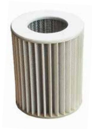
The cartridges are **used to filter Natural Gas, refinery gas, propane, air and other non-aggressive gases**. They have an high filtering capacity and great accumulating capacity; the filtering fabric is BIA-USGC certified, and it is thermostabilized from the input side for better removal of powders. They protect gas regulating and measuring equipment from mechanical erosion by powders. They are suitable for 100% Hydrogen in case the contamination of H<sub>2</sub>S is =<1%.
