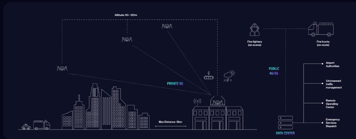
The drones have been successfully linked to Verdi and Frontforce, the fire department's dispatching systems. This allows the safety drone to be placed in the call train between the regular vehicles. This ensures that the safety drone can be called without any additional action being required from the fire department personnel.
