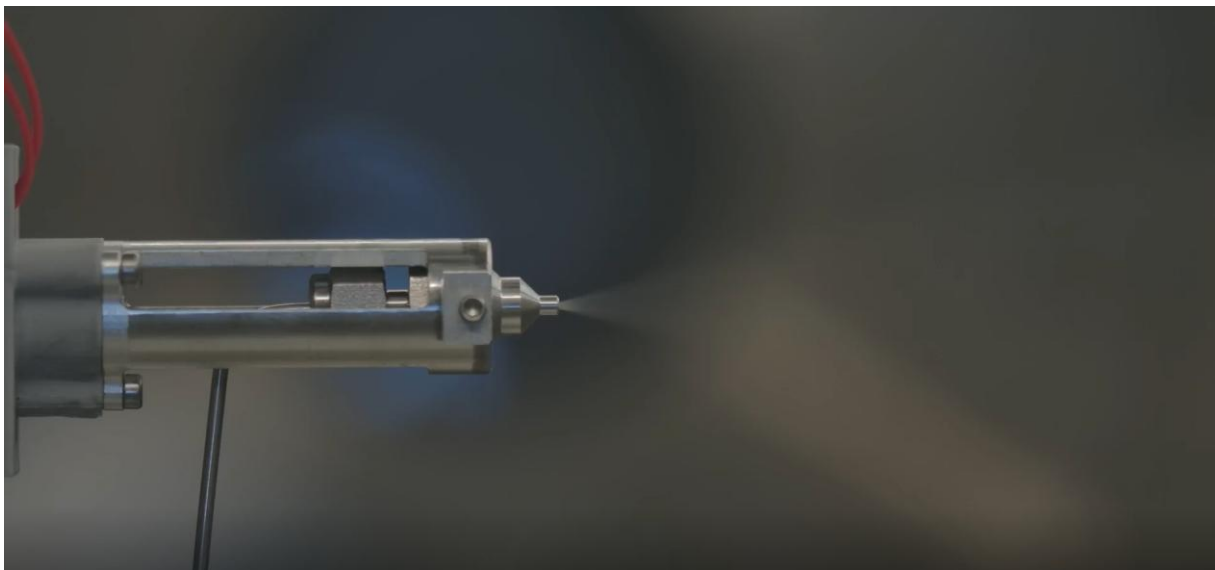
Figure 1: Cold gas thruster during testing
