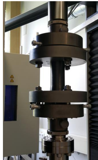
ZWICK universal testing machine Z250 with climate chamber
