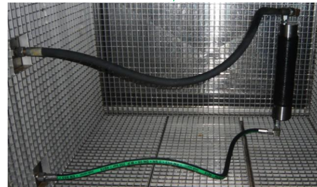
test rig with climate chamber for inner pressure
