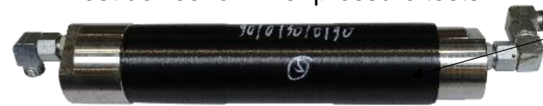
Test device for inner pressure tests
