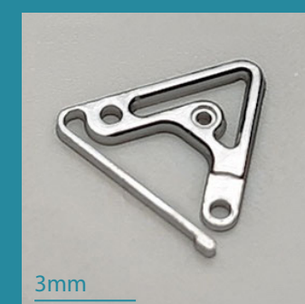
Example of a micromechanical part made using microthermomolding
