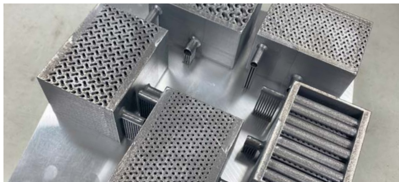
Additive manufactured metal heat exchangers
