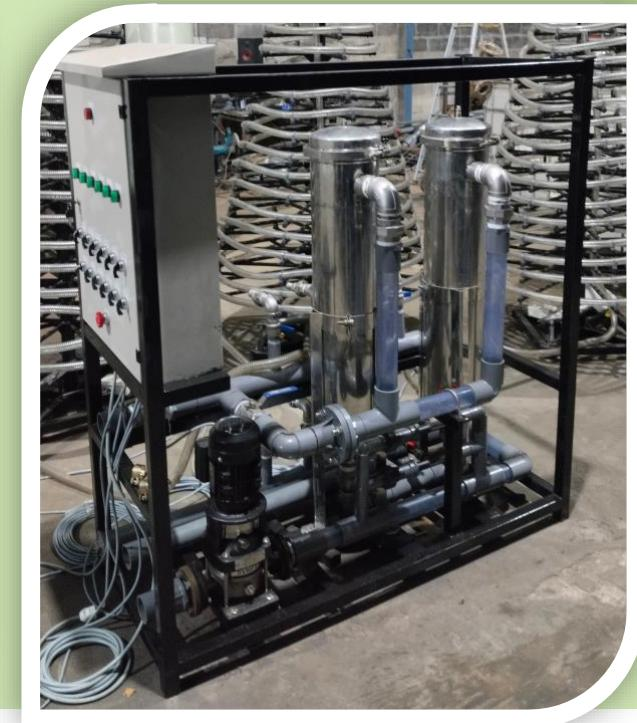
**A closed-loop bioreactor** system designed to convert aquaculture wastewater into natural fertilizer for seaweed and microalgae cultivation.
