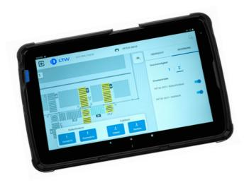
In addition to controlling our stacker cranes using a stationary HMI, there is now the convenient option of operating them directly on site using a mobile tablet. The advantage is that the operator can move anywhere they want to in the warehouse and has a clear overview of any faults that occur on the usual user interface, the LIOS Cockpit. This lets them keep a constant eye on the entire system visualization and can address issues as effectively as possible.
