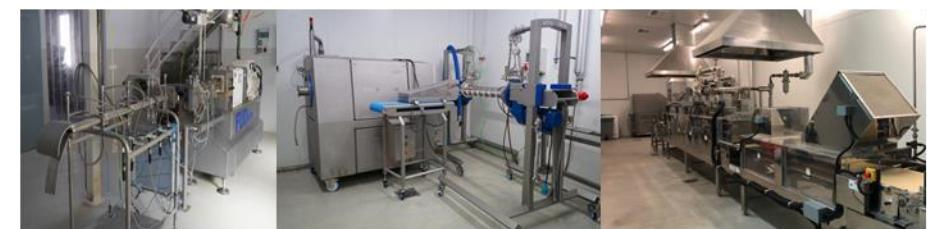
Dry/HME/cooking extrusion: 4x pilot extruders
