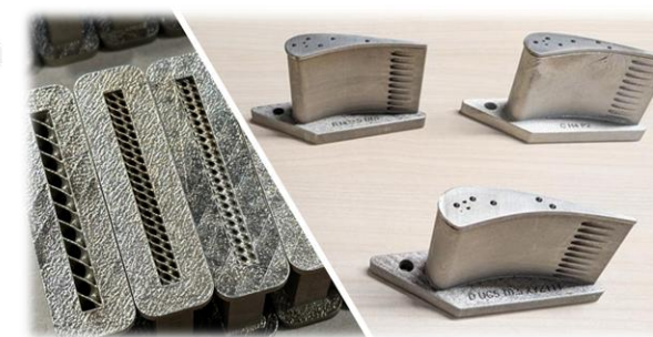
3D printed cooling systems (coupon and gas turbine vanes)
