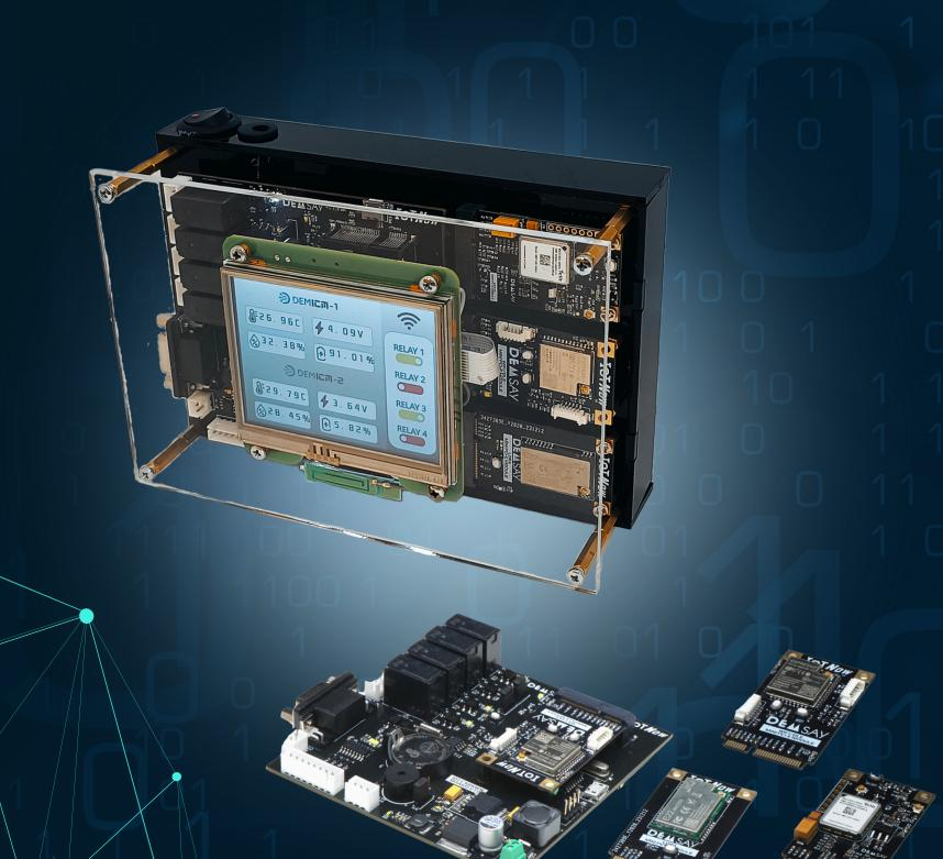
THE IOT CARRIER BOARD IS DESIGNED FOR USE IN INDUSTRIAL WIRELESS COMMUNICATION PROJECTS. WITH SUPPORT FOR MINI PCI-E COMPATIBLE MODULES, IT PROVIDES CONNECTIVITY FOR THE MPCIE FORM 2G-NB IOT CATM1 + GPS/GNSS GSM MODULE AND BLE-WIFI MODULE. IT FEATURES 4 RELAY OUTPUTS, RS232 CONNECTION, EXTERNAL UFL ANTENNA CONNECTION, ISOLATED POWER INPUT SUPPORTING UP TO 40V, AND A MICRO USB CONNECTION.
