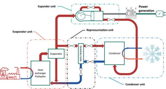
The cycle uses ammonia (R717). A natural, high-performance fluid that is not harmful to the environment but has toxicity constraints.
