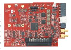
mixer and FIR filter. The generated error signal is directly applied to the laser current, ensuring stable laser frequency.
