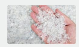
Transparent PET classified through grinding, washing and drying is produced into high-purity flakes.
