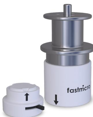
The Fastmicro Surface Particle Sampling Kit introduces a new, optimized sampling method that improves both cost-efficient and consistent surface particle sampling. The kit includes a sampling tool designed for fixed-force application to ensure repeatability and prevent cross-contamination, along with a sample holder that is backward-compatible with existing Fastmicro Sample Scanners.
