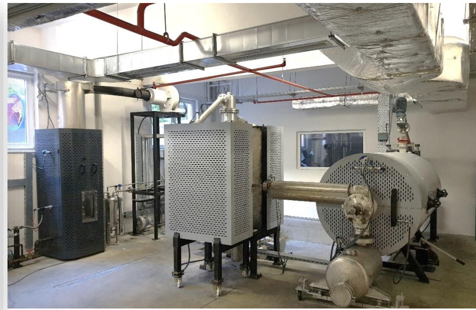
Pilot Scale Pyrolysis and Gas Clean-Up High temperature continuous pyrolysis unit with 15-20 kg/h feed
