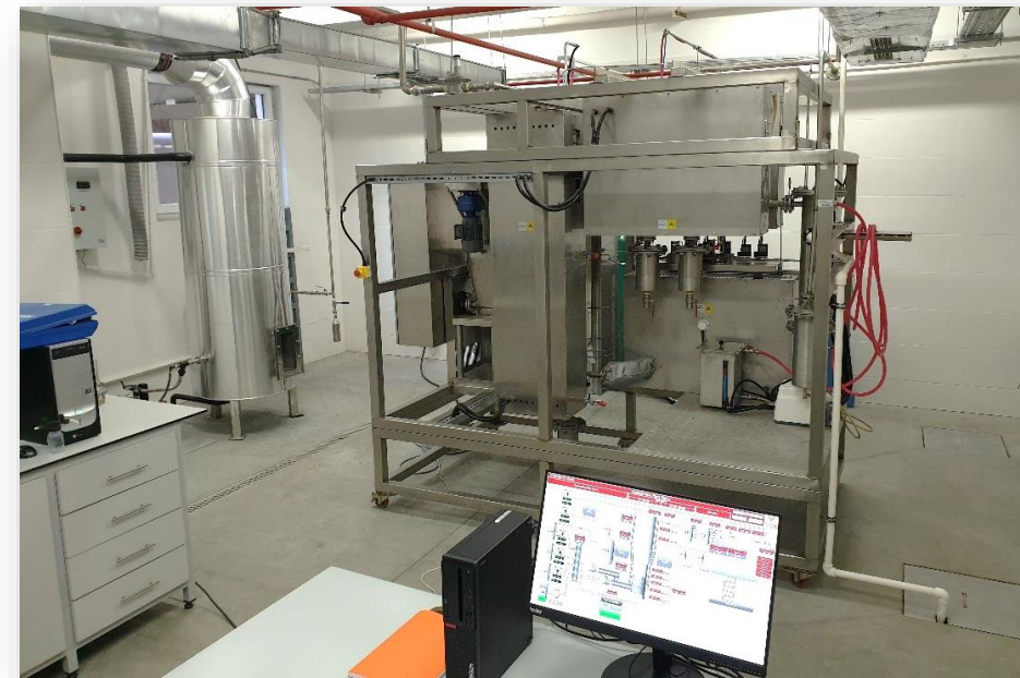
Semi Pilot Gasification and Gas Clean-Up Continuous fluidized bed gasification unit with 5 kg/h feed and flare system
