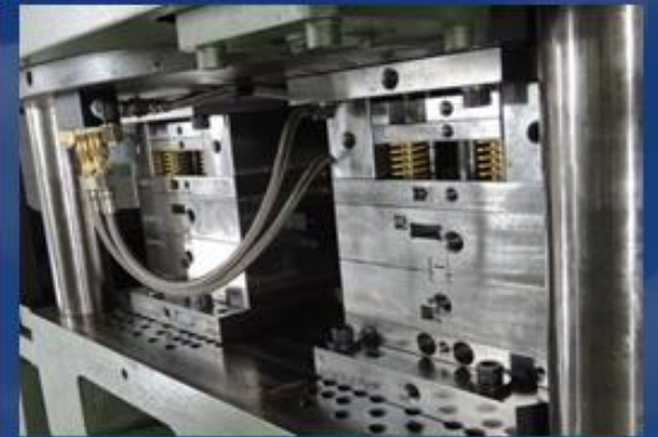
One Color Plastic (ABS) with One Color Transparent Plastic (ABS, PC, Acrylic) 2 Shot Injection
