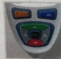
Figure 1. This dashboard controller is a clamshell design, the lower half being a two-shot part. The primary shot on the lower part of the body is PC/ABS, and the second shot is a seal in TPE. The upper portion of the controller (the part that is invisible in the picture) is a single-shot part also in PC/ABS. The keys are made using the in-mold design (IMD) process. The keys are printed, thermoformed, trimmed, and back injected with PC/ABS. The film is PC. The final step in the process is insert molding the single-shot top. The keys are then inserted into the mold, and a TPE seal is molded around them (this is the gray material between the keys and the white top). The TPE is flexible enough to allow the keys to be depressed to activate the audiovisual system in the room. This is a good example of creative use of IMD being integrated into an active portion of the product. The key tops are durable and bright, and the graphics are behind a protective layer of polycarbonate. The final operation of insert molding the keys on the body is an elegant way of providing good key travel and a water-resistant interface. (Source: Yomura)
