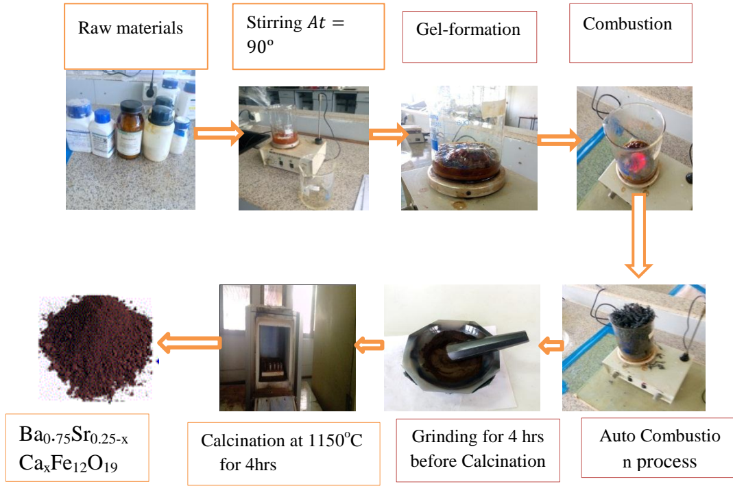
Figure 3.4: Producers for synthesis of \text{Ba}_{0.75}\text{Sr}_{0.25-x}\text{Ca}_x\text{Fe}_{12}\text{O}_{19} hexaferrites (Misbah et al., 2022)
