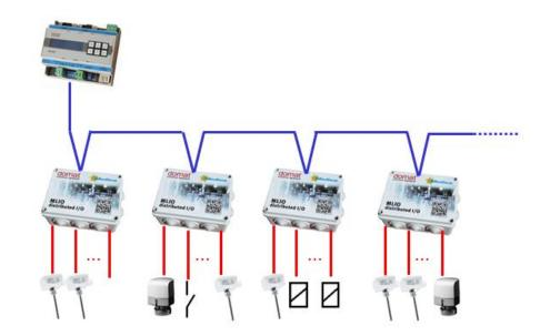
Together with the MLIO modules, there may be other module types on the bus, room units, variable speed drives etc., communicating Modbus RTU. However, separate buses for modules installed in the cabinet and outside the cabinet are recommended: with a common bus for all modules a and short-circuit of the bus in the field, the communication with the modules in the cabinet would be broken.
