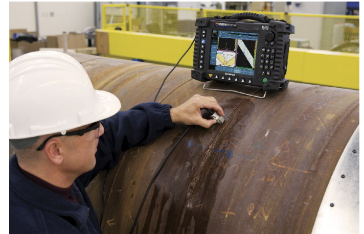
NDT Testing for pipeline inspection (on-site)
