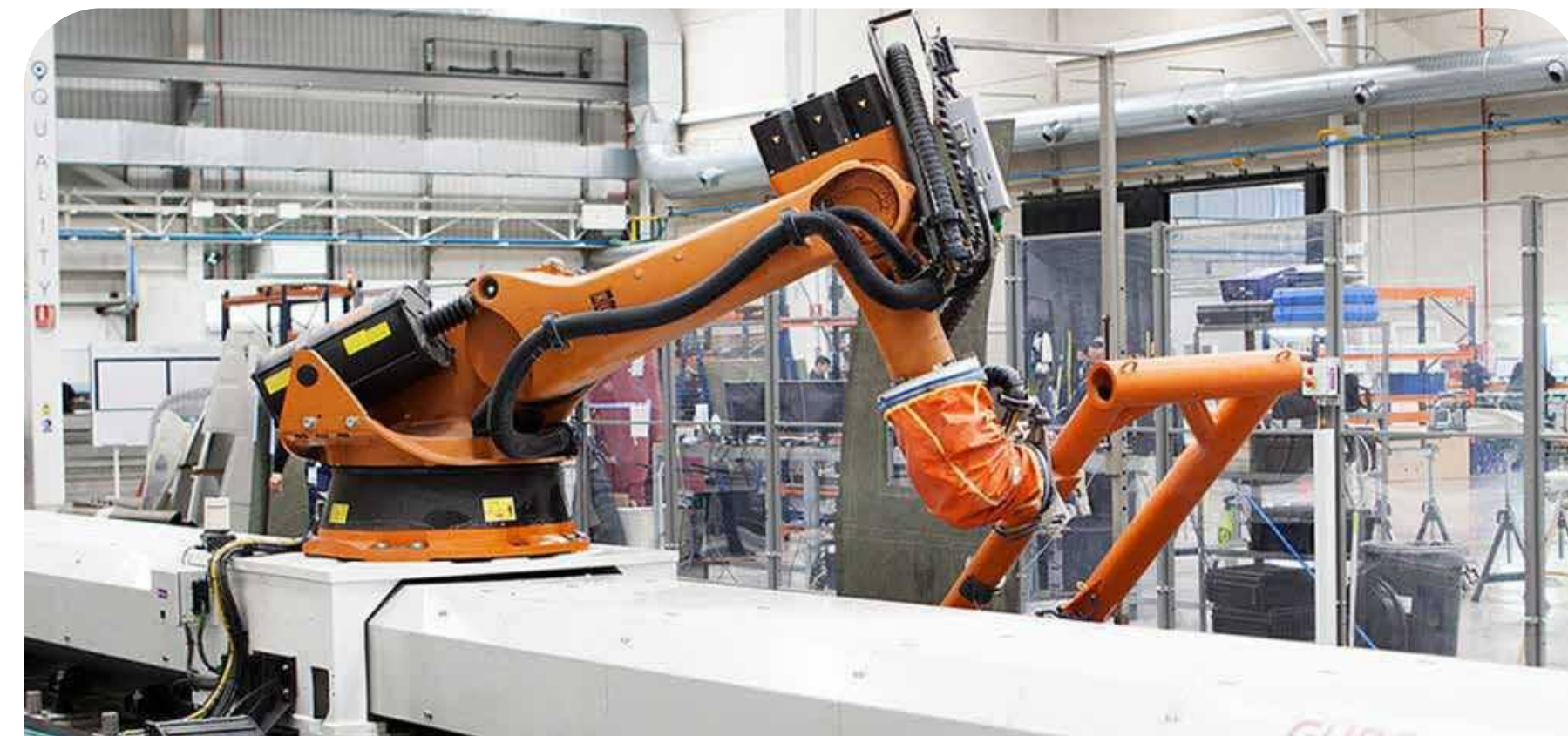
ROBOT AUTOMATIC TRANSMISSION - PHASE-ARRAY - A/B/C SCAN 14 x 2,5 m. / 40 x 8 ft
