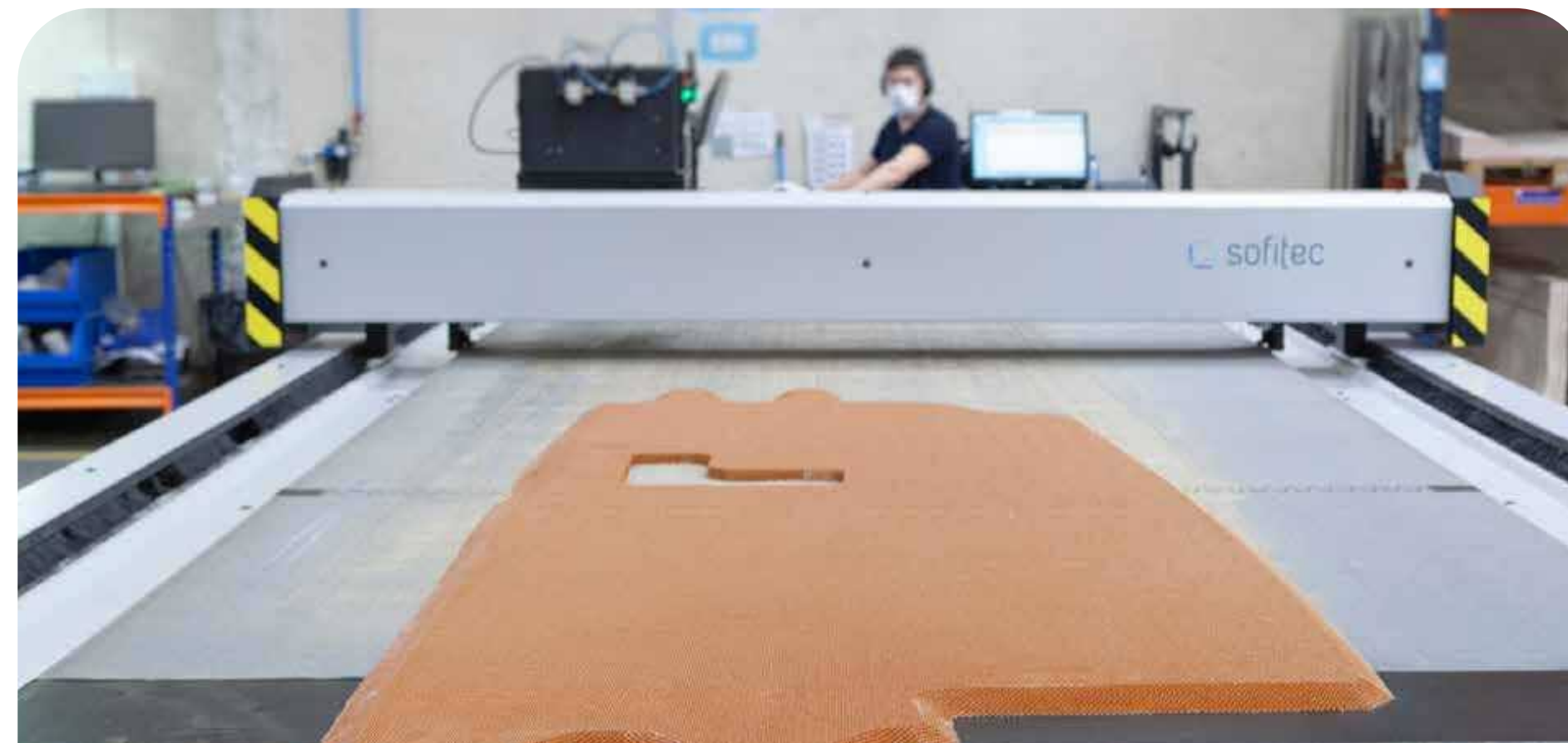
HONEYCOMB TRIMMING & CHAMFERING 10x3,6 m. / 32x12 ft
