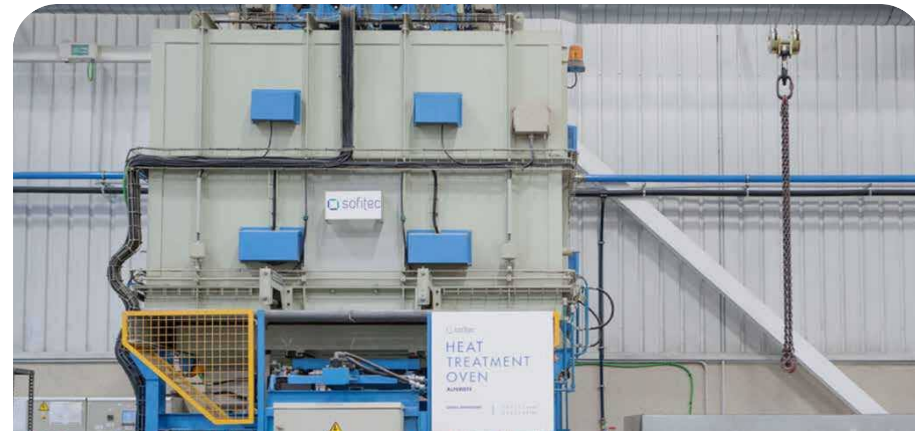
HEAT TREATMENT OVEN 1800x1000x1000 m m. / 6 x3.3x3.3 ft. (WxHxL)
