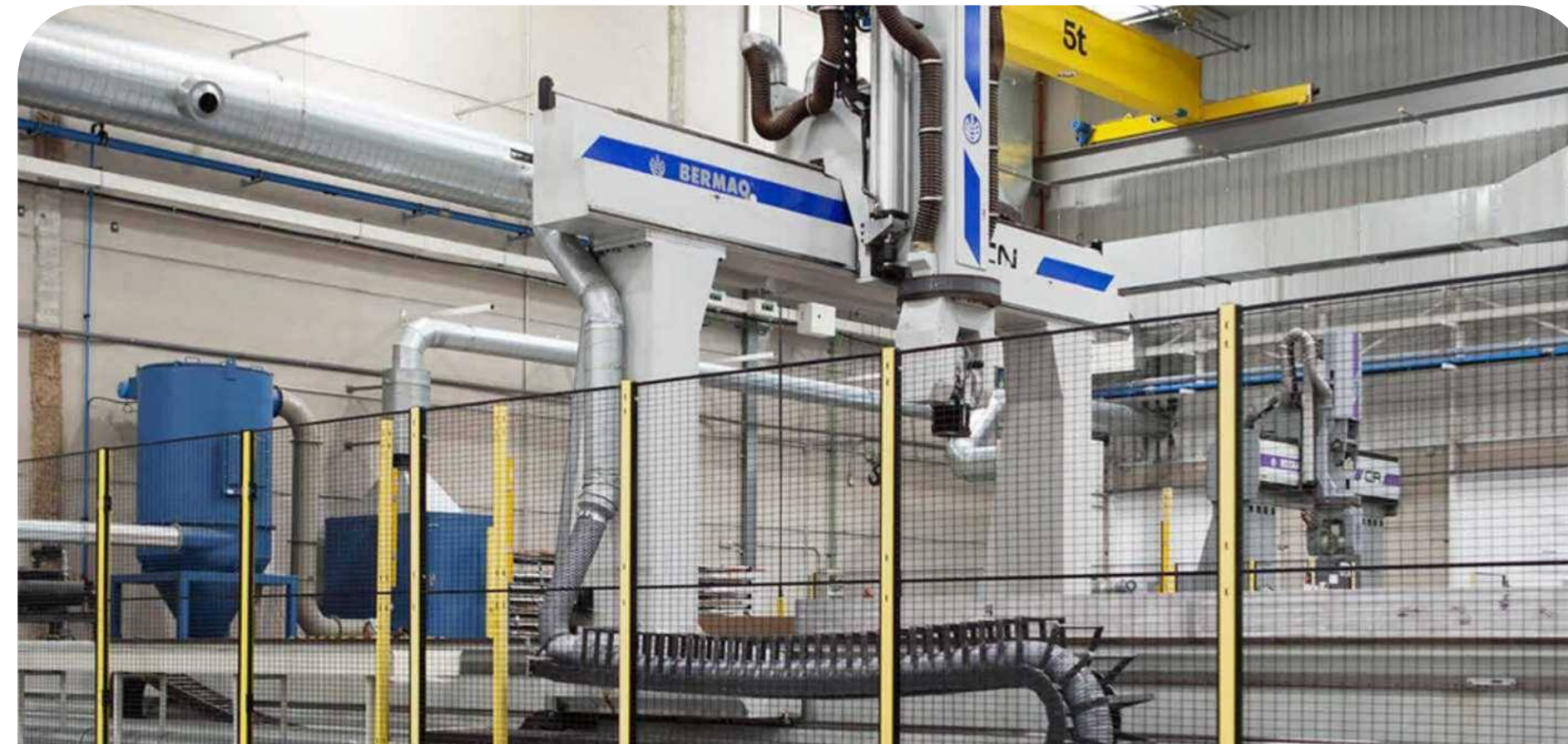
5X CNC 13x4x1.1 m. / 43x13x3.6 ft (LxWxH) COOL JET REGRIGATION
