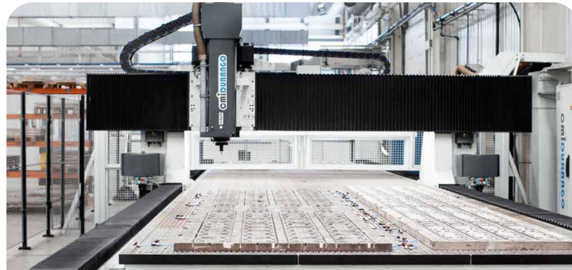
3X CNC 14x3x0.35 m. / 46x10x1.15 ft (LxWxH) 2 WORKING ZONES / MQL & COOL JET REGRIGATION
