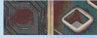
Blind hole on the silicon substrate (side of 50μm and the depth of 80μm)
