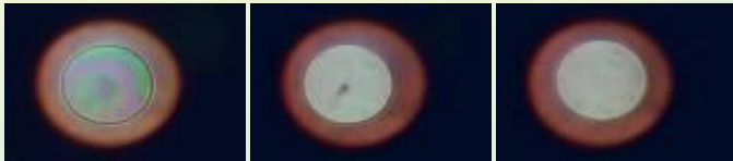
Laser removal of a film of photoresist ( 2 \mu\text{m} thick) from silicon substrate
