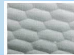
Microlens arrays 22x22 \mu m, 216.8 \mu m pitch
