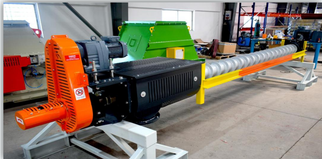
Water-cooled Screw Conveyors For Ash Extraction
