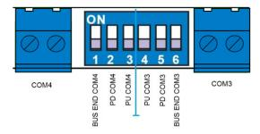
Unlike at the older PLC versions, the RS485 buses are separated from each other. It is possible to activate all PU and PD switches at the same time.
