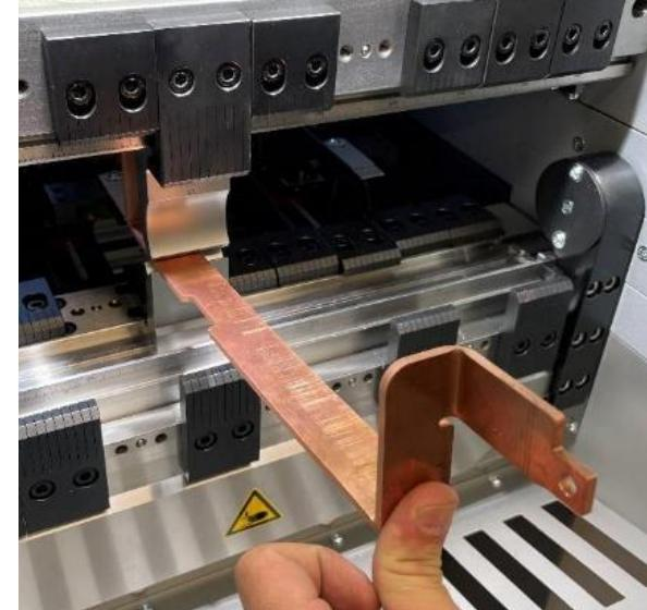
Copper Busbars up to 5mm thickness
