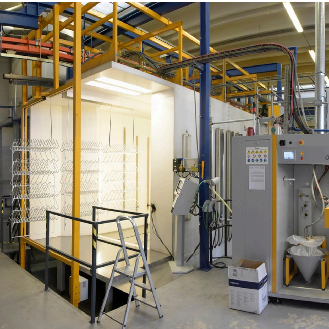
SURFACE FINISHING Automatic Continuous Powder Painting Line max. 3.000 x 1.800 x 1.500 mm
