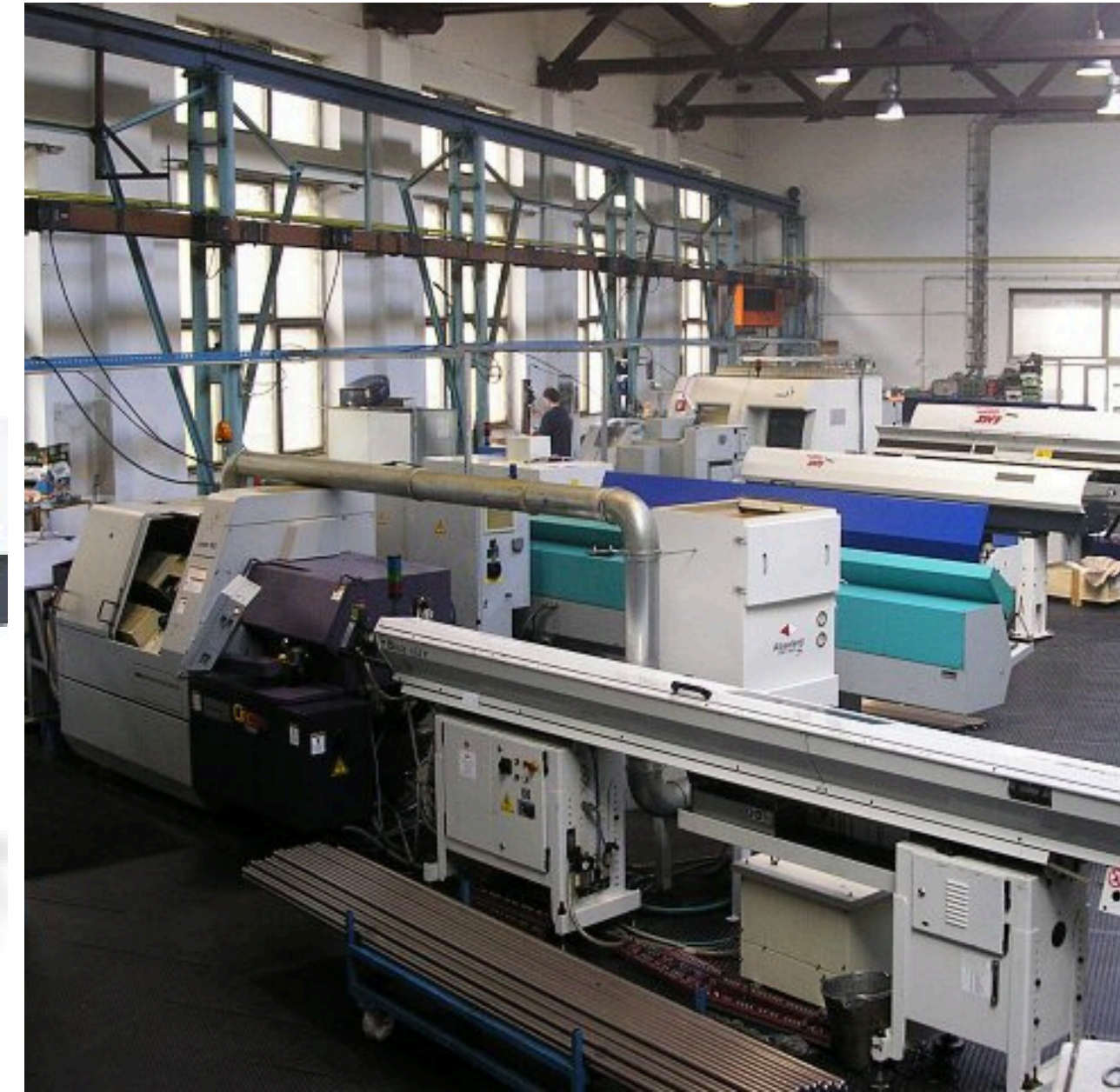
CNC TURNING dia. 2 - 60 mm from 3.000 mm bars max. dia. 500 mm from cut piece
