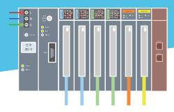
The PLC PLUS gateway module captures input and output communication from the PLC controller to collect production data. Emulation of the HMI signal allows users to operate the PLC through a virtual HMI on a computer and add customized controls. Previously undisplayed data, such as data from management systems, can also be shown on the virtual HMI to facilitate on-site operations.
