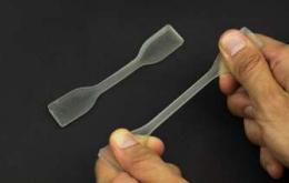
**Biosourced & recyclable shape memory elastomer from hydroxylated fatty acids.** Breaking strength (10 mm/min): approximately 2 MPa. Elongation at break (10 mm/min): 150 - 250 %. - Solvent- and chain-blocker-free process.
