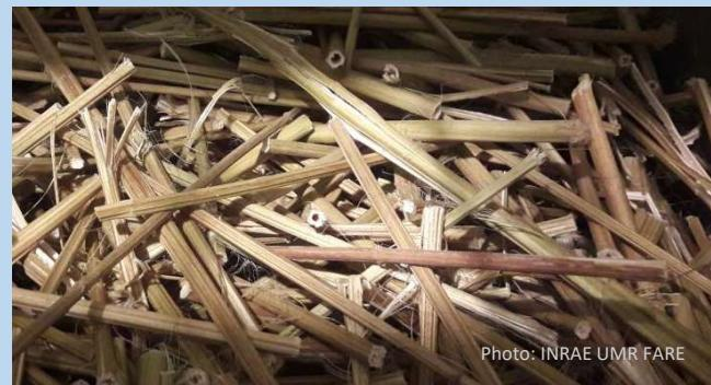
**4FM - FARE & FRD-LAB** common laboratory for Future Fibres and Materials (FRD) aims to validate the results of projects carried out jointly by FRD and UMR FARE in an operational situation on the scale of Europe's largest hemp production basin. Hemp concrete was first used in house construction in 1986. Hemp shives are the fundamental ingredients in this biobased concrete. INRAE partnership with company FRD to improve the quality of hemp shives as well as that of other plant fibres.
