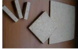
**Agromaterials production by bioextrusion of a solid lignocellulosic material seeded with fungal biomass;** low density for building materials, packaging, thermal insulation, or high density after thermopressing.
