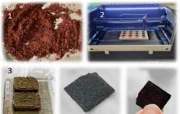
**Biobased composite powders (10-200 microns) for additive manufacturing (selective laser sintering 3D printing) of materials.** Modulation of the final properties by formulation (% PHA, waxes and lignocellulosic fillers).
