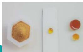
**Biobased furylated polyphenols: custom-made functionalized platform molecules for speciality chemistry (resin, hardner agent).** One-step, low-pollution, soft conditions production process from Douglas fir bark.
