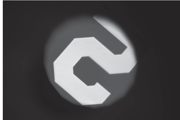
Epi-illumination image at the same magnification, showing adjustable illuminated area (approx. 0.1-2mm) for optimizing spatial resolution and signal throughput in reflectance measurements.
