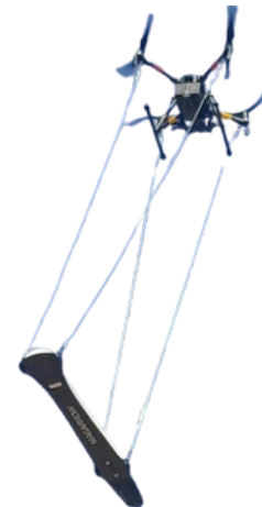
Automated data collection via UAV and Airborne Magnetometer
