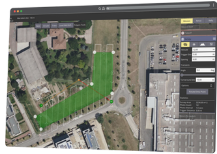
Interface for configuring automated flight missions.
