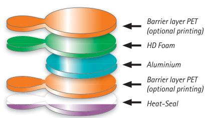
With the tab now not effecting the induction process, **ALKOflex™** tab can be any size or shape, allowing it to be consumer friendly whilst ensuring a hermetic sealing all the time.
