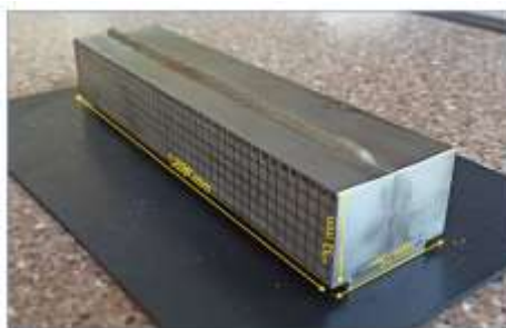
Figure 1. General view on the sample of the electron beam welded joint in EUROFER97
