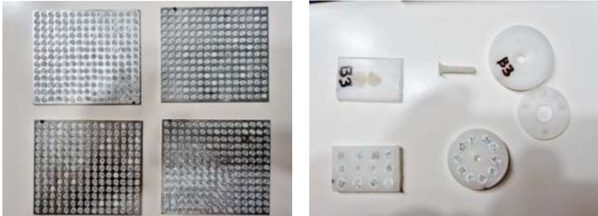
Fig. 1 (Left) Image of detectors prepared for the annealing process, (Right) Components of boxes with detectors. The boxes filled with detectors were screwed to the plugs.
