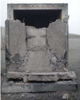
Experimental (top) and numerical (bottom) damage on concrete structure of a charge at distance
