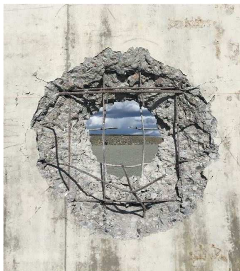
Experimental (left) and numerical (right) damage on concrete structure of a charge in direct contact
