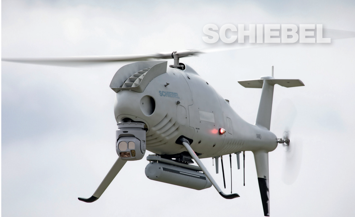
CAMCOPTER® S-100 equipped with EO/IR, Radar and Mobile Phone Detector
