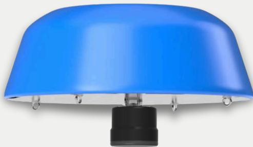
**MEDUSA PING** is a buoyant device equipped with lithium-ion batteries, offering an autonomy of up to 30 days. It features an echo sounder capable of measuring depths ranging from 0.50 m to 100 m with a 25-degree beam angle.
