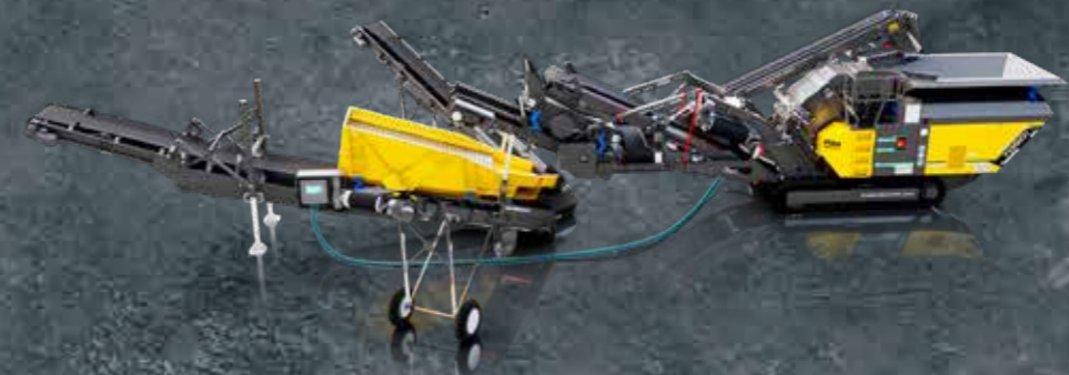
RM 7060! 2.0 COMPACT CRUSHER POWERS RM CS3600 COMPACT SCREEN ATTACHMENT
